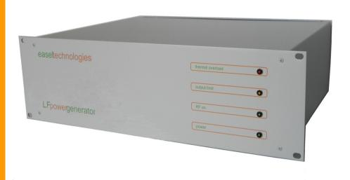
easel technologies' low frequency generator is versatile, efficient and robust. It provides up to 300W over the frequency range 90kHz to 450kHz and is designed to cope with high VSWR loads typical of demanding applications such as plasma processing.
